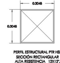
**COLUMNA METÁLICA C4.**
