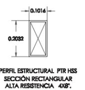
**COLUMNA METÁLICA C3.**
